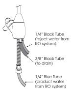
Be sure faucet spout and body are in position, and align the slotted washer and spacer to allow access to hose barbs. Tighten the hex nut while holding the faucet in position with a padded crescent wrench. Do not over tighten.
