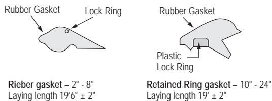
Gasketed pipe offers low assembly force; flexibility to allow for variations in line pressure and changing working conditions; compensation for movement due to thermal expansion and contraction; a certain amount of allowable joint deflection; and positive, leak-free seals for both high- and low-pressure applications as well as vacuum service.
