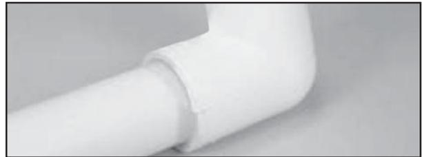
Any cement, in excess of the bead, can be wiped off with a dry, clean rag.
