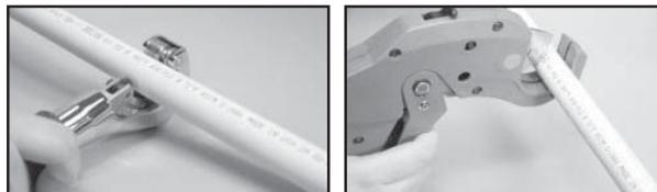
Be careful not to split the tube if using a ratchet-type cutter, especially in temperatures below 50°F. If any damage or cracking is evident, cut off at least 2" of the pipe beyond any visible crack.
