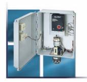
These controls combine an AquaMatic stager with a reliable Autotrol® timer, mounted and prewired in a NEMA-rated enclosure. Stagers are initiated by timeclock or impulse controls. The cycle times are programmable to accommodate a wide range of applications.
